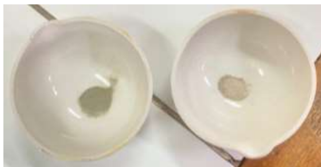
Figure 1. Comparison of SnO 2 powders before furnace heating (left) and after calcination (right).
