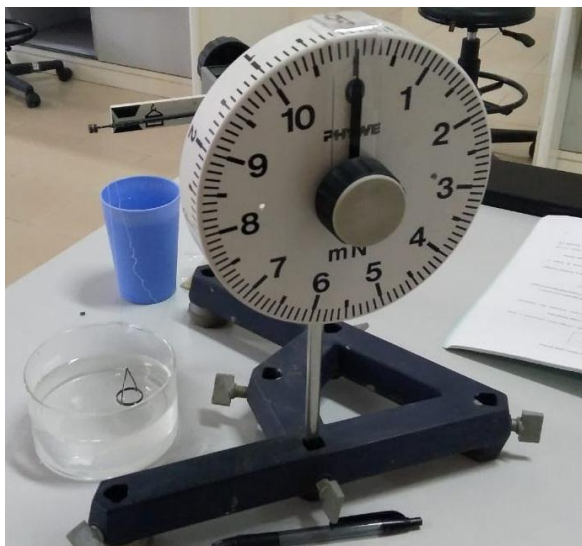
Figure 1. Photo of team practicum fisika dasar (2016) on torsion dynamometer.
