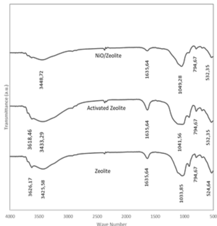
Figure 2: FTIR Spectra of Zeolite, Activated Zeolite, & NiO/Zeolite
