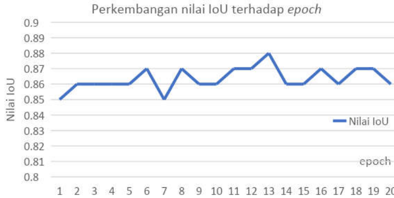
Figure 9. Graph of IoU values of test data against epoch
