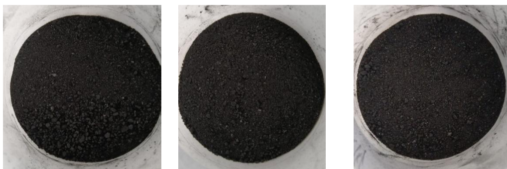
Figure 5. Activated Carbon at Carbonization Temperature of 500°C with HCl, KOH, and ZnCl 2 Activation
