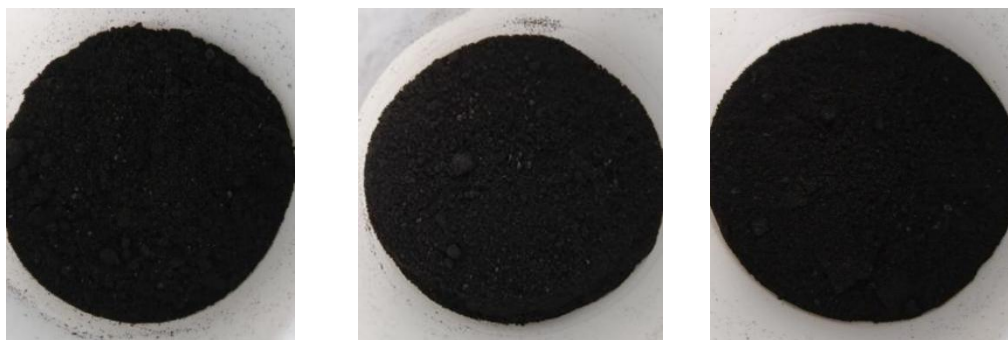
Figure 3. Activated Carbon at Carbonization Temperature of 300°C with HCl, KOH, and ZnCl 2 Activation
