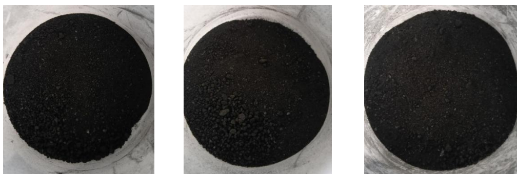
Figure 4. Activated Carbon at Carbonization Temperature of 400°C with HCl, KOH, and ZnCl 2 Activation
