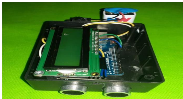
Figure 4. Display of digital distance measurement instrument based on Arduino Uno
