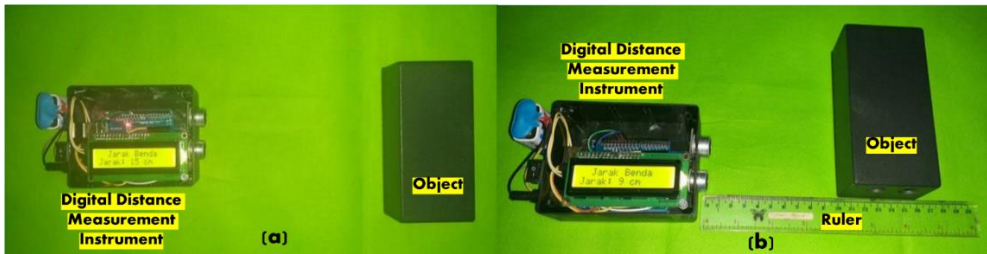
Figure 5. (a) display of object distance measurement and (b) display of comparison of distance measurement instrument digitally with a ruler
