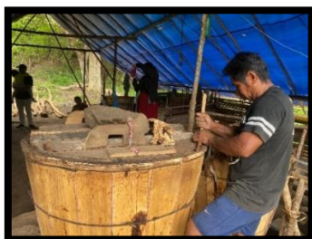
Figure 7. Installing the Kettle Lid Process
